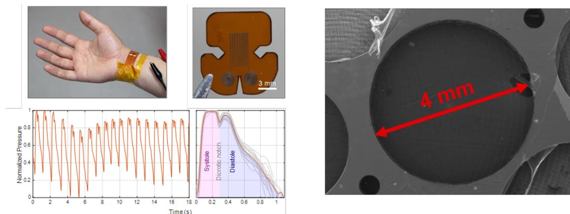
**Fig. 1** Left: LIG strain gauges used in the measurement of the arterial pressure waveform and an example of data collected. Right: few-layered 4 mm wide graphene membrane.
