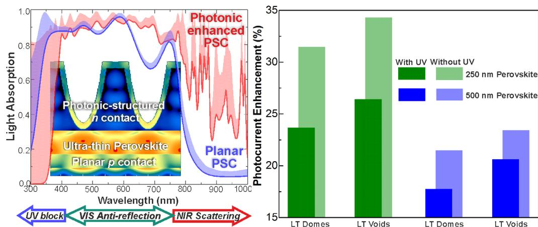
**Fig. 1.** Left - simulated light absorption profile for the best LT case in Perovskite solar cells. Right - photocurrent enhancements attained with the two types of optimized LT structures based on TiO<sub>2</sub> voids or domes arrays, relative to the planar reference cells.
