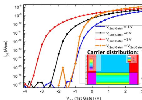
**Fig. 1.** Simulation of a dual-gate TFT showing the effect of biasing conditions for the second-gate.
