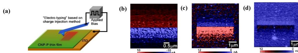
**Fig. 1.** (a) Schematic of charge injection through AFM probe. (b) Visualization of current mapping during charge injection with different bias voltage (from  $\pm 1$  to  $\pm 7$ V). Visualization of current mapping after charge injection using (c) +5V and (d) +1V bias voltage.
