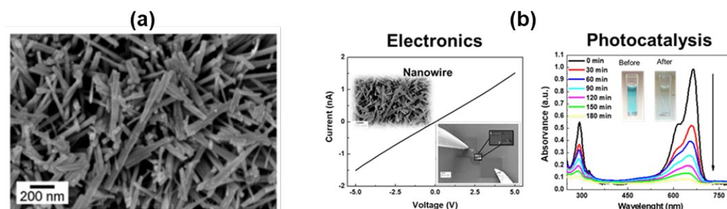
**Fig. 1.** (a) SEM images of the fabricated  $\text{ZnSnO}_3$  nanowires. (b) Examples of applications explored (electronics and photocatalysis).
