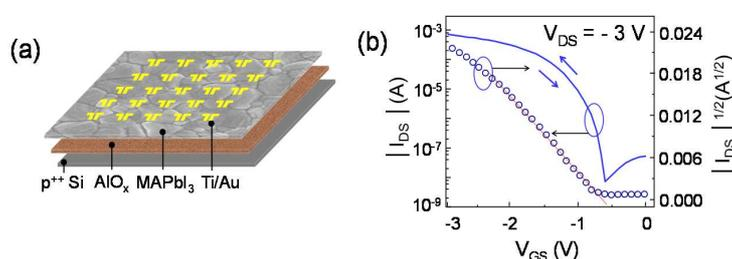
**Fig. 1.** (a) Schematic of TFT showing the Ti/Au Drain Source metal contacts, deposited via shadow masks; the MAPbI<sub>3</sub> as semiconducting channel. Transfer characteristics (module of  $I_{DS}$  and  $I_{DS}^{1/2}$  vs  $V_{GS}$  at constant  $V_{DS} = -3$  V) of MAPbI<sub>3</sub>-DES based TFT.
