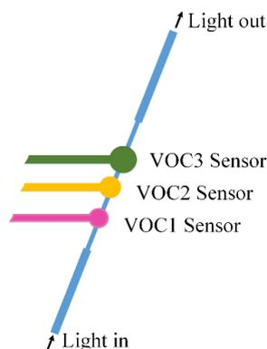
**Fig. 1.** Schematic design of the proposed lab-on-fibre scheme, based on three microspheres coupled to a fibre taper.
