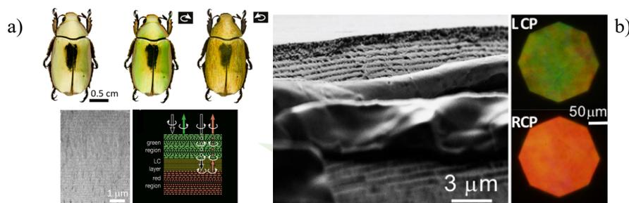
**Fig. 1.** a) *Chrysina resplendens* beetle observed at normal, left-handed and right-handed polarized light bottom TEM-image of the beetles exocuticle<sup>1</sup>. b) SEM image of a cross-section of the bio-inspired CNC film with a micro-gap filled with 4CB, where top and bottom cholesteric domains have different pitch sizes (left). Optical images of left- and right-handed circularly polarized light reflectance of a CNC/5CB composite system (right).<sup>2</sup>
