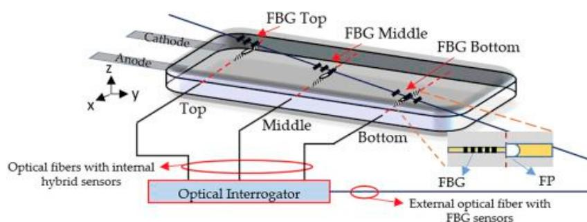
**Fig. 1.** Intergration of optical fiber sensors in Li-ion batteries to monitor characteristic parameters.
