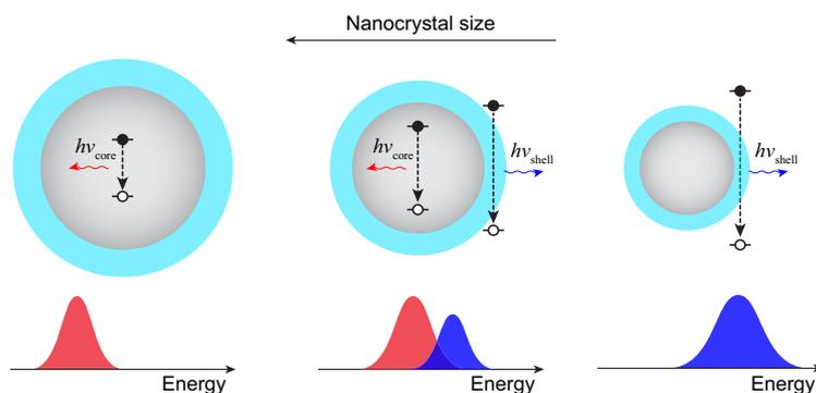
**Fig. 1.** Size-dependence of the origin of light emission in surface-oxidized Si-NPs.
