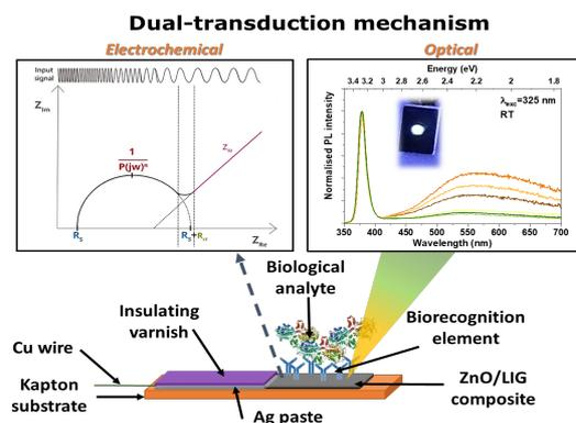
Fig. 1. Schematic representation of the main objective of the project: dual-transduction biosensors.
