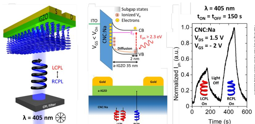
Fig. 1. Device representation and mechanism of CPL sensing with  $\lambda=405$  nm.
