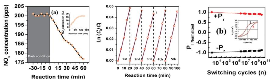
**Fig. 1** (a) PCA abatement of  $\text{NO}_x$  gas by a 3-layered Aurivillius ferroelectric. (b) Fatigue resistance of 5-layered Aurivillius thin film up to  $10^{10}$  cycles, 1 and 2 represent switching before and after fatigue.
