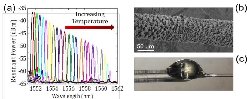
**Fig. 1.** (a) Thermal calibration of a FBG; (b) SEM image of a polymeric fibre core damaged by fuse effect; (c) Microscope image of the developed magnetic field sensor.
