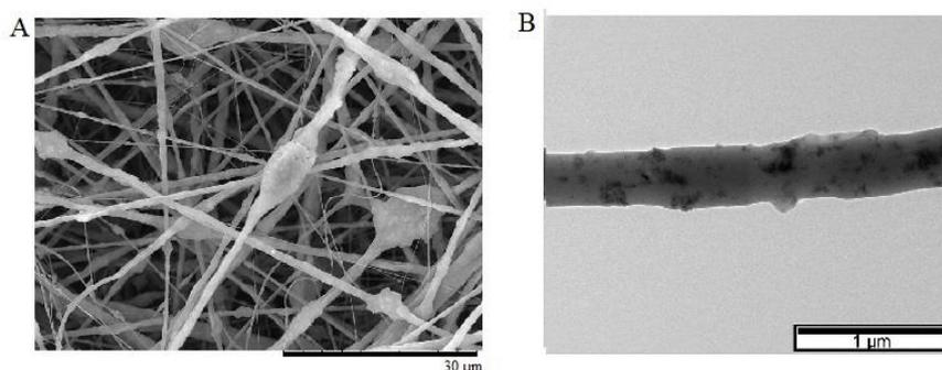
**Fig. 1.** SEM image of PVP/MBG 80S15 composite (A) and TEM image of PVP/SPIONs (B).
