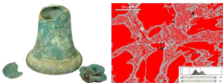
**Fig. 1.** Image of Coruche bell and OM image of its bronze microstructure (red: Cu rich-phase; grey:  $\text{Cu}_3\text{Sn}_8$ -phase; white: Pb; black: pores).
